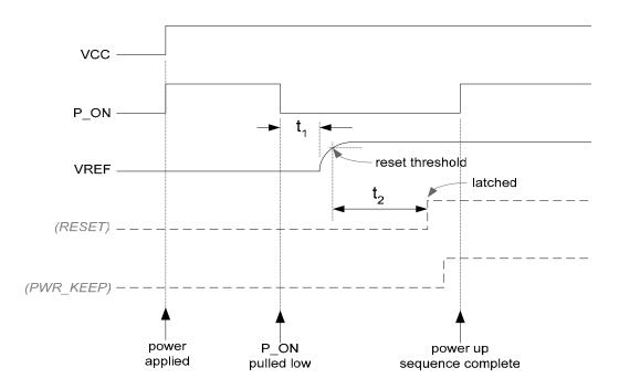
Figure 5.8-2 Power On timing using PON\_L as an example
